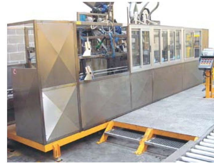
PA-30-TA Automatic filling machine for 5 to 60 litres.
