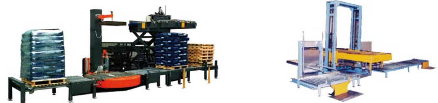
HB-600: Low load palletisers for boxes, sacks or bundles.
