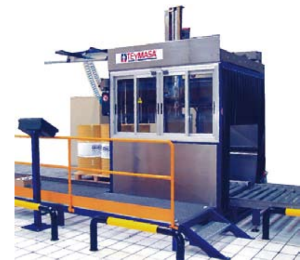
PST-1001: Automatic filling on pallet. Automatic introduction and extraction of pallet. Positioning of axes using CTM -Control Through Memorisation - with AV -Artificial Vision- option for searching for orifices.
