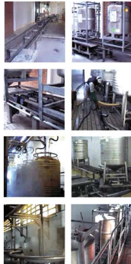
Management system of metal containers for internal and external cleaning.
