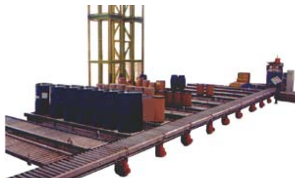
Accumulation system for grouping waste into different families before sending it for grinding and combustion.
