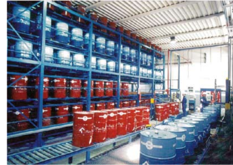
SAT-5 Automatic storage for empty drums with capacity for 1,200 drums.
