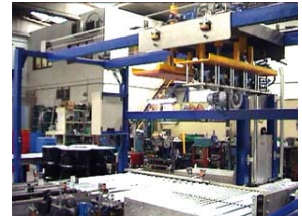
PBC-200: Automatic palleting of drums, kegs, cylinders and tanks at several levels.
