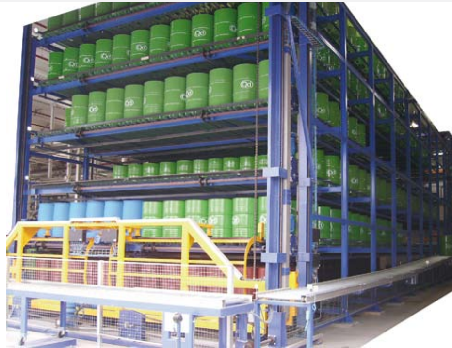
SAT-6 Automatic storage for empty drums with capacity for 1,944 drums.
