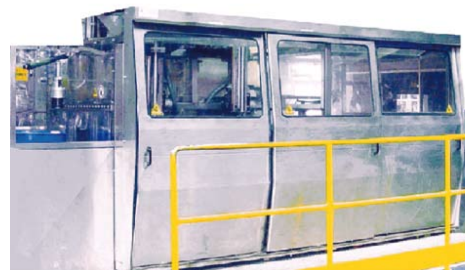
PA-200-TA: In-line filling with automatic uncapping and capping.
