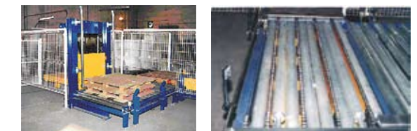
Pallet distributor and chain changer.
