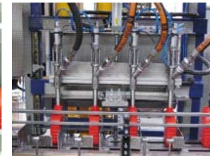
Filling module with 4 filling stations.
