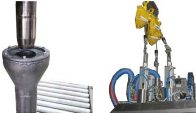
Cleaning cone for reducing the generation of waste in the cleaning process of lines and diverse tubes in machines always connected to the input of the product to prevent spills and stoppages.
