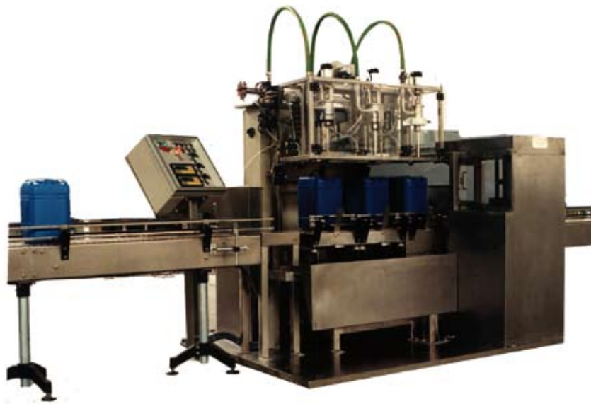
PA-30 weight control filling machine.
